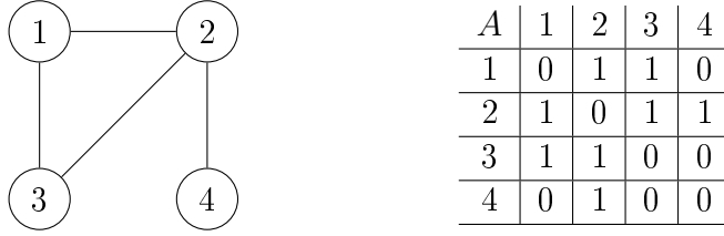
Figure 4: The same undirected graph in graphical (on the left) and adjacency matrix (on the right) representations.
