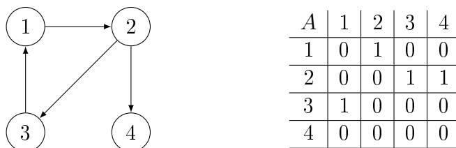
Figure 3: The same digraph in graphical (on the left) and adjacency matrix (on the right) representations.
