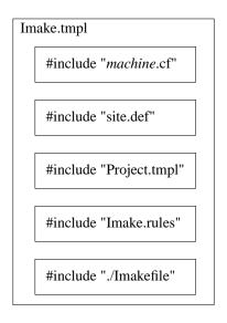
**Figure 4:** structure of *imake* template used by X
